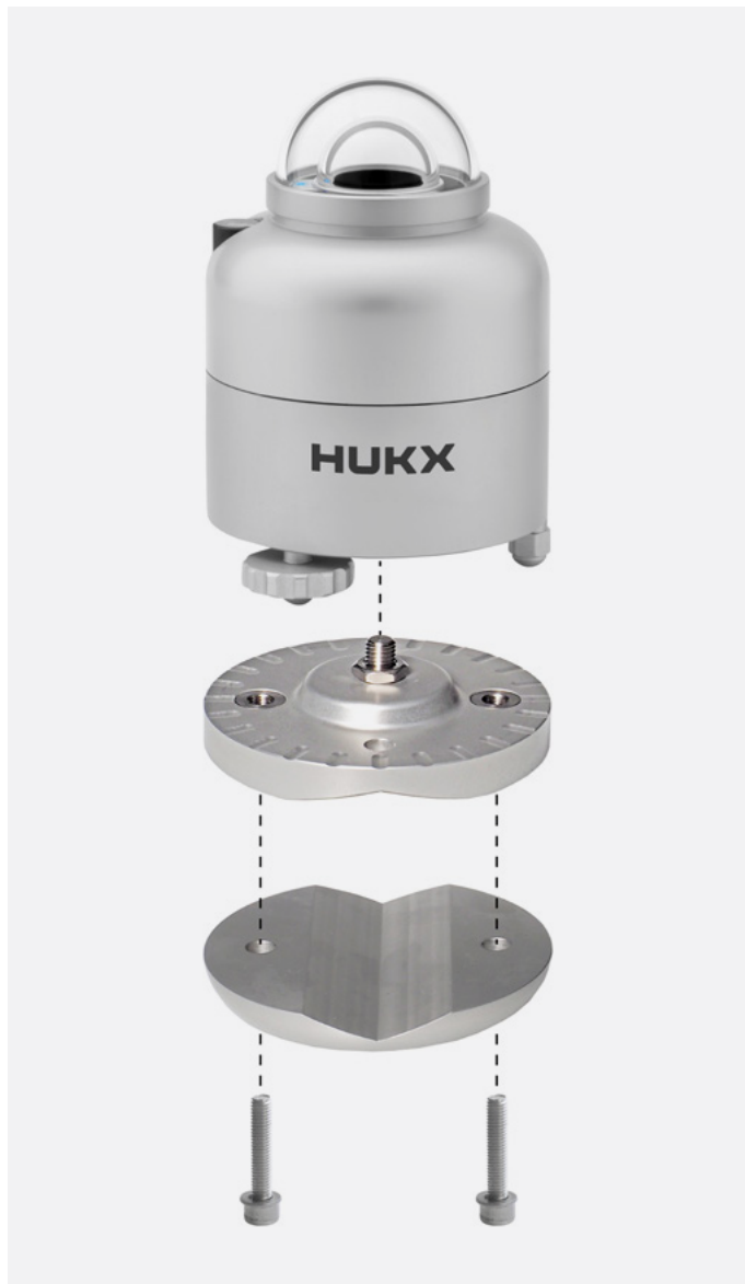
Figure 7 Optional LM01 spring-loaded leveling mount (one part) and TLM01 tube leveling mount (2 parts) for SR300-D1. Spring-loaded leveling is a major time-saver during installation.
