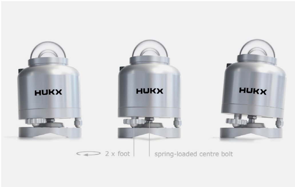
Figure 5.3.6.1.5 Pyranometer locked on its optional leveling mount: by fastening (on the left) or loosening (on the right) the two adjustable feet, the pyranometer can be levelled, using the bubble level as a reference.
