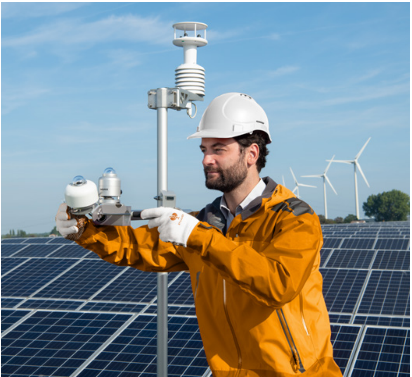
Figure 0.2 SR300-D1 includes a digital tilt angle measurement, a practical feature for remote verification of instrument mounting orientation. The above image depicts two SR300-D1 pyranometers, one tilted for Plane of Array (POA) measurement, and another mounted horizontally for Global Horizontal Irradiance (GHI) measurement.
