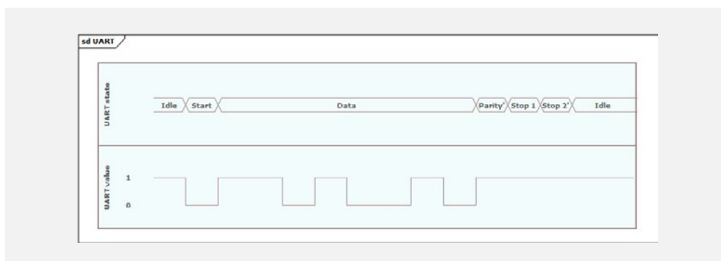
Figure 1.1.1 An example UART frame.
