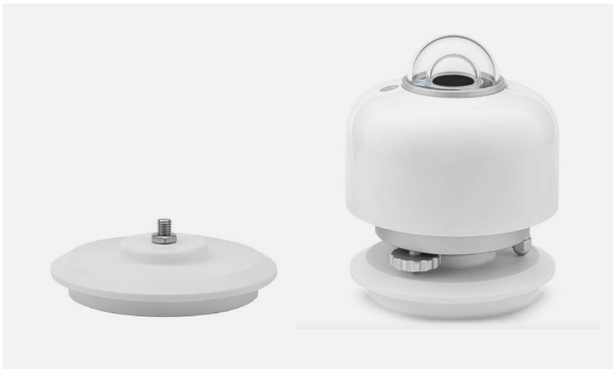
Figure 3 The PID01 Pyranometer Insulation Disk. On the right, SR300-D1 mounted on a PID01. Also visible: one SF static foot and one LF leveling foot.
