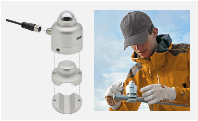
Figure 4 The Class C model SR05 is smaller than the Class A and B pyranometers and has slightly different mounting and leveling. The optional ball leveling and tube mount, TMBL01 (including BL01), allow for easy installation, leveling, and removal.
