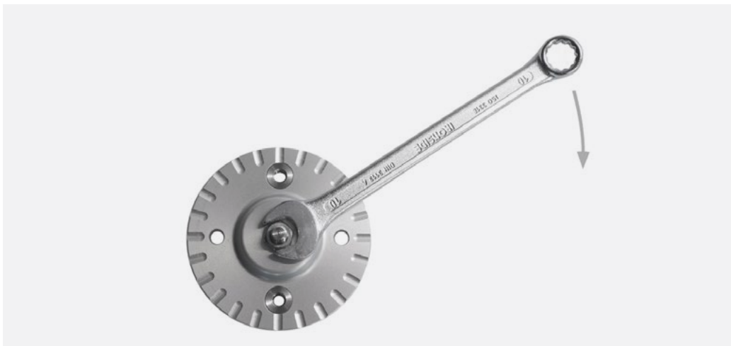
Figure 5.3.4.1.3 LM01 leveling mount seen from above: (un) locking with a 10 mm spanner.
