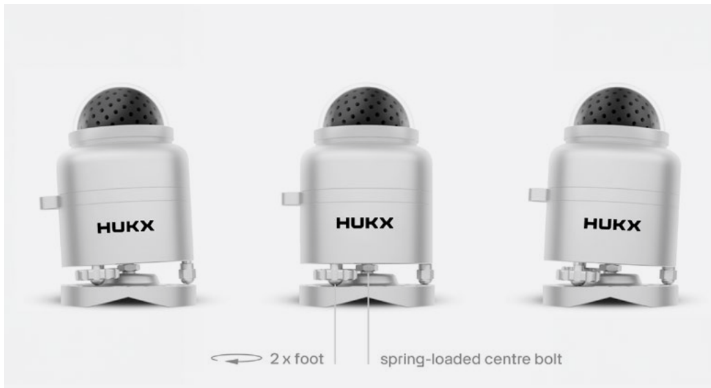
Figure 5.3.4.1.5 SRD100-D1 locked on its optional leveling mount: by fastening (on the left) or loosening (on the right) the two adjustable feet, the pyranometer can be levelled, using the bubble level as a reference. The static foot remains fixed. In all cases, ensure the legs of the pyranometer fit into one of the small ledges of the leveling mount. Locking is in place, when the nut is turned all the way against the bottom plate of the pyranometer.
