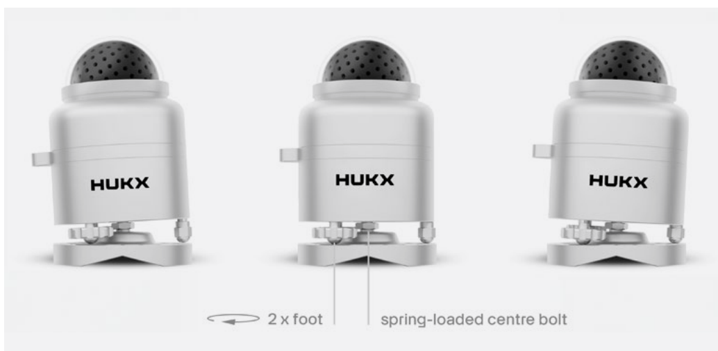
Figure 0.8 LM01 leveling mount is the most popular option for SRD100-D1: practical spring-loaded mount for easy mounting, leveling and instrument exchange on flat surfaces. The spring-loaded mounting has the advantage that leveling can be done quickly, without unlocking the instrument.
