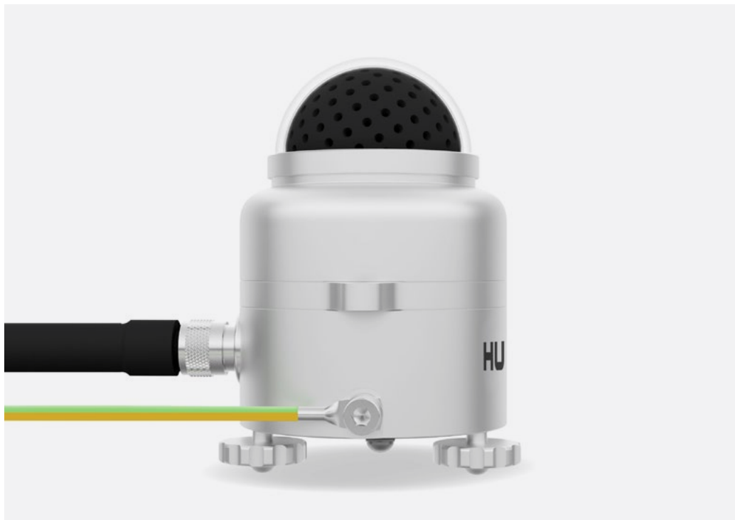
Figure 0.5 SRD100-D1 with yellow/green wire connected to its earthing terminal for compliance with EU and US safety regulations.
