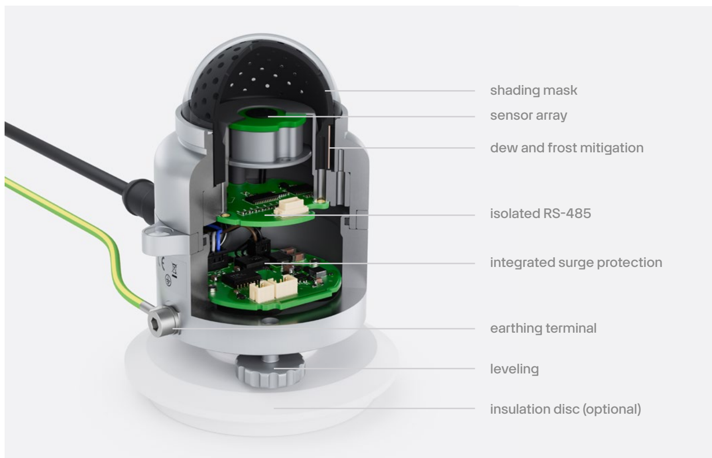
Figure 0.2 Inside the SRD100-D1 diffusometer: a detailed look at the core components responsible for performance and durability under extreme conditions.
