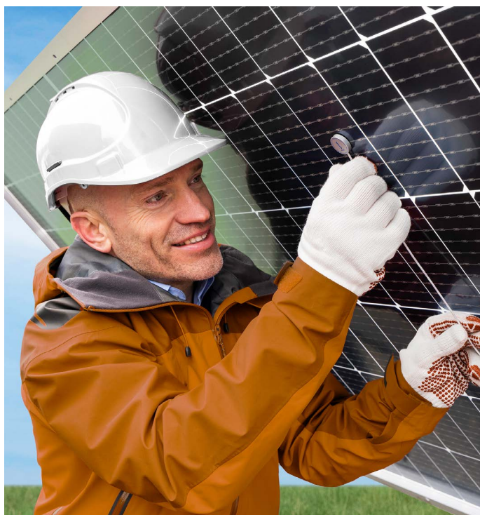
Figure 3 PVMT01 installed on the rear side of a PV module. The sensors are preferably installed at the center of a cell, close to the center of the module. IEC requires 3 sensors per monitoring station
