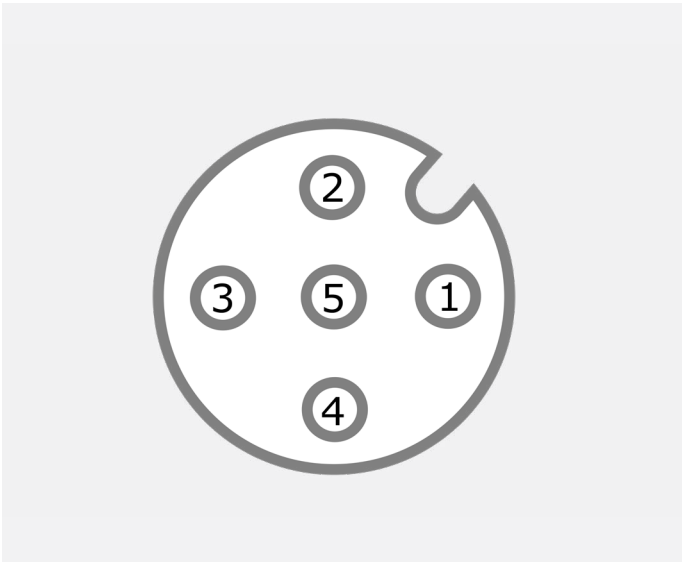
Figure 4.2.2. Schematic of the extension cable M12-A connector layout, indicating the pin numbers.
