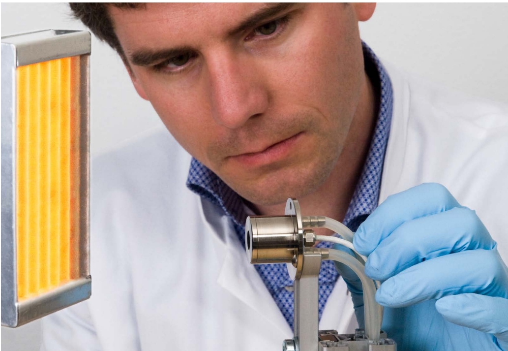
Figure 1.3 SBG01 is the sensor of choice for fire testing.
