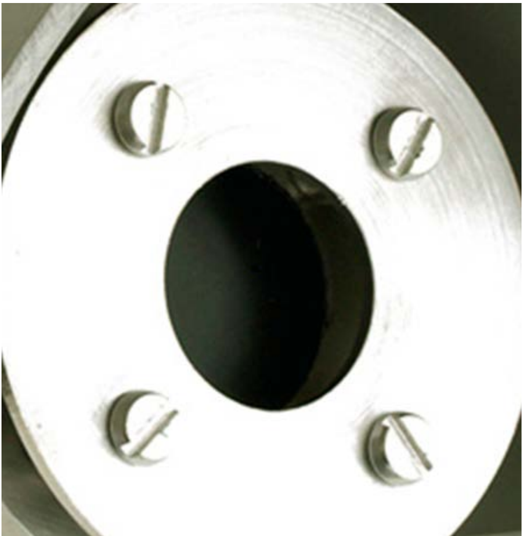
Figure 6.11 Picture of HF02's sensor surface. The sensor surface should be inspected on a weekly basis. The picture shows that the sensor field of view is unobstructed, and that the sensor surface is not scratched and that it is clean.
